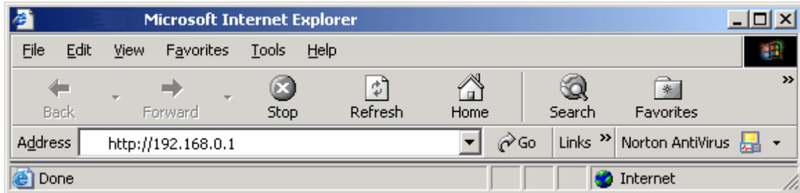
First connect to the Actiontec® DSL Modem using your Web browser [Internet Explorer]. In the address bar enter `http://192.168.0.1` and hit Enter on the keyboard.
